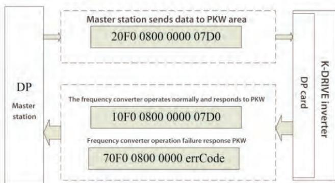
Figure 2-10 Example of master station reading frequency converter parameters and sending PKW data
