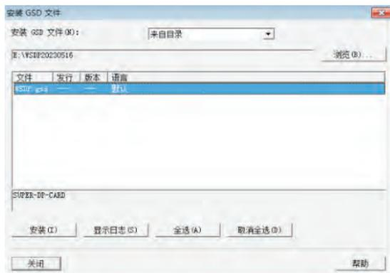
Click Install, and after installation is completed, the Profibus-DP module for SUPER-DP-CARD will exist, as shown in the following figure.
