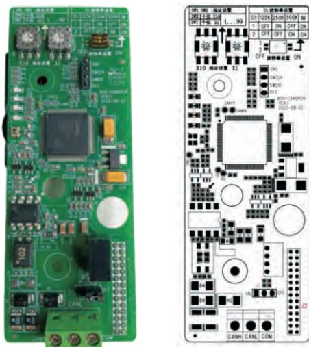
Figure 2-13 Layout diagram of CAN communication card
