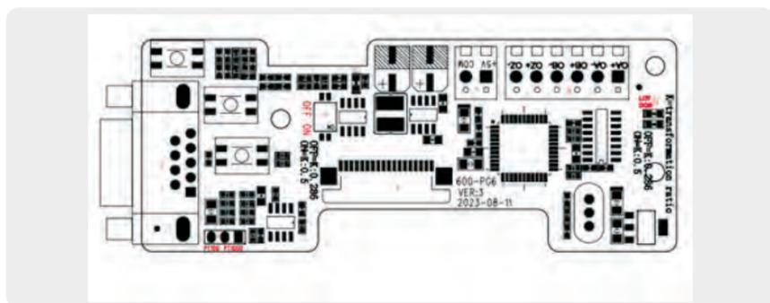
Figure 3-6 PG6 Rotary transformer interface card appearance
