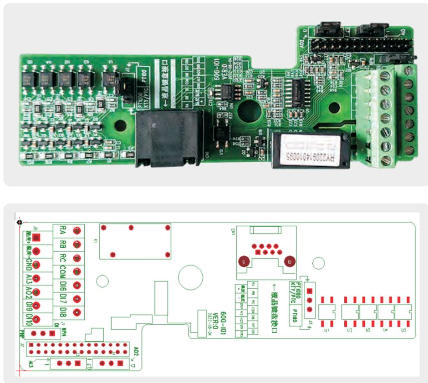
Figure 1-1 I/O Expansion Card 1 Appearance and Layout
