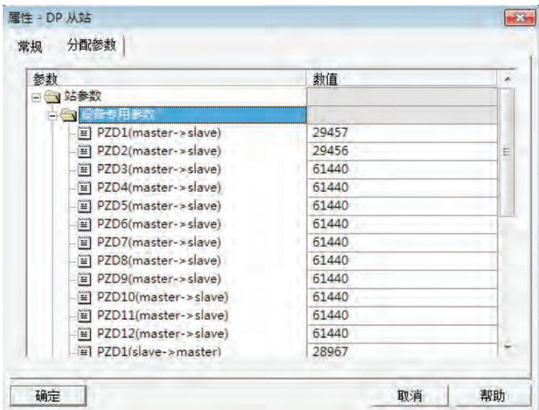
Among them, PZDx (master -->slave) represents the corresponding address written by the master station to the slave station, and PZDx (slave -->master) represents the corresponding address read by the master station to the slave station. The PZD range that can be set is PZD3~PZD12, and the display format is decimal. That is, if you want to set PZD3 (master -->slave) to P0-12, you need to fill in 61452 in the value of this line.
