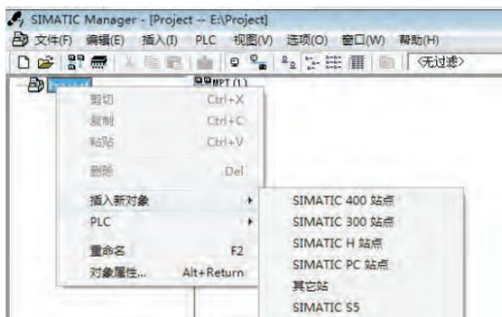
2. Double click on the hardware icon to enter HW config configuration, and add WSDP in the HW config configuration screen GSD file, the operation is as follows (note: GSD file should not be stored in the Chinese path, otherwise Step7 may not recognize it):
