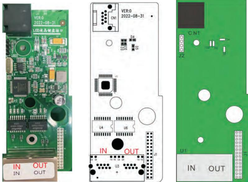
Figure 2-11 Ethercat communication card Card Appearance and Interface Layout
