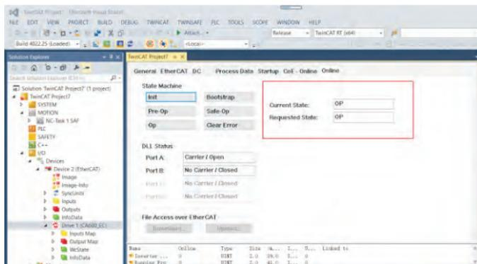
5. Control communication drive through PDO. Write the corresponding value through the configured RPDO to control the AC drive.
