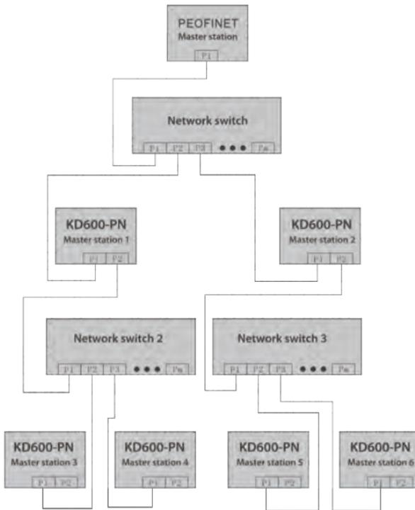
Figure 2-4 Tree connection topology diagram
