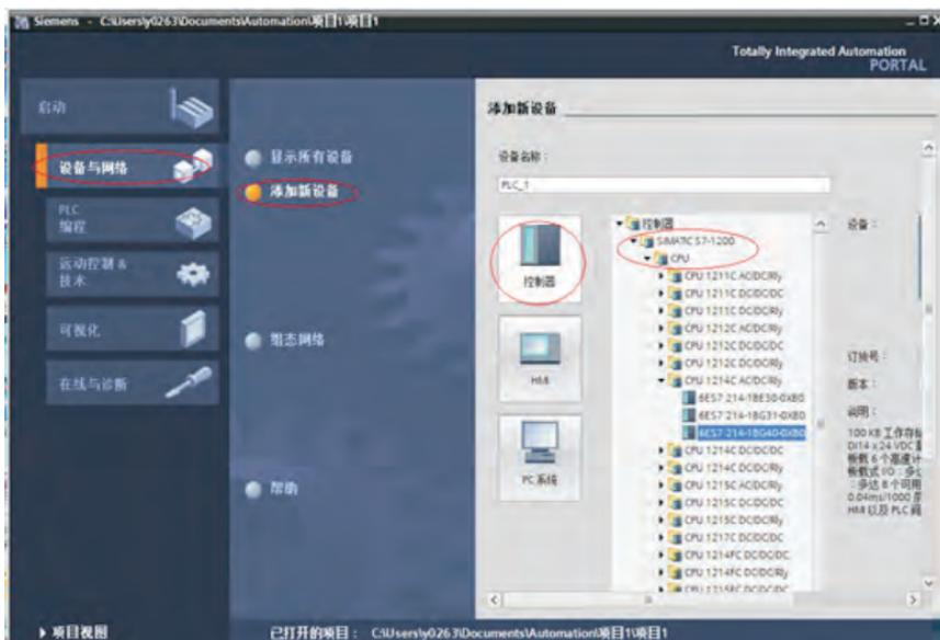
After adding Siemens PLC, switch to the "Project View".
