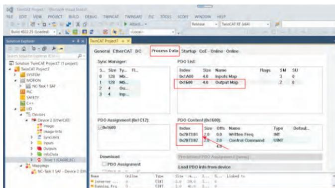
3. View the SDO data list. After the OP status is activated, you can view real-time data in the SDO data list or double-click the object dictionary to modify SDO data.
