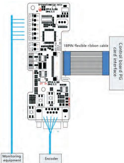
Function Description of Rotary Transformer Interface Card Terminals
