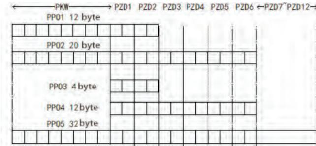
Figure 2-5 PPO type data format
