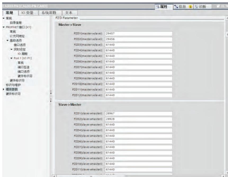
Among them, PZDx (master -->slave) represents the corresponding address written by the master station to the slave station, and PZDx (slave -->master) represents the corresponding address read by the master station to the slave station. The PZD range that can be set is PZD3~PZD12 (depending on the selected message type), and the display format is decimal. That is, if you want to set PZD3 (master -->slave) to P0-12, you need to fill in 61452 in the numerical value of this line.
