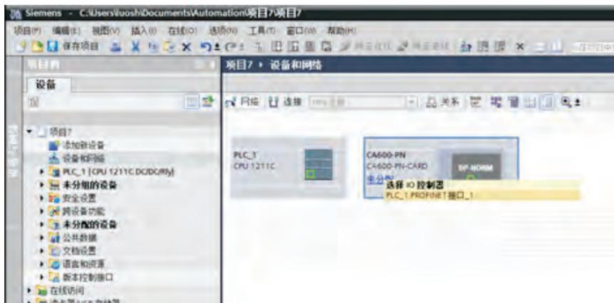
(2) Double click the \_ PN icon to enter the configuration module, select the appropriate PPO type in the "Hardware Directory", pay attention to the addresses assigned to each segment, as shown in the figure below. Mark the corresponding PKW addresses in the marked section. If the selected PPO does not have a PKW, the column will be blank.
