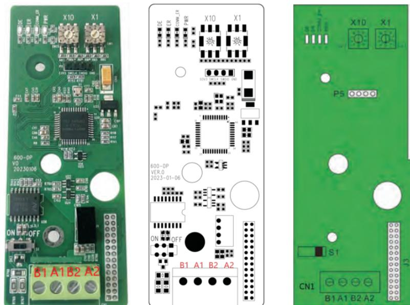
Figure 2-7 Profibus-DP Communication Card Appearance and Interface Layout
