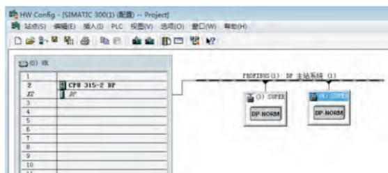
In the above figure, Station 4 is SUPER-DP for comparison purposes only, without detailed explanation. SUPER-DP and this DP expansion card can coexist simultaneously in the same network.
