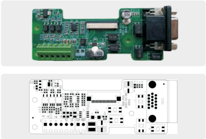
Figure 3-5 Appearance diagram of PG5 sine cosine encoder interface card
