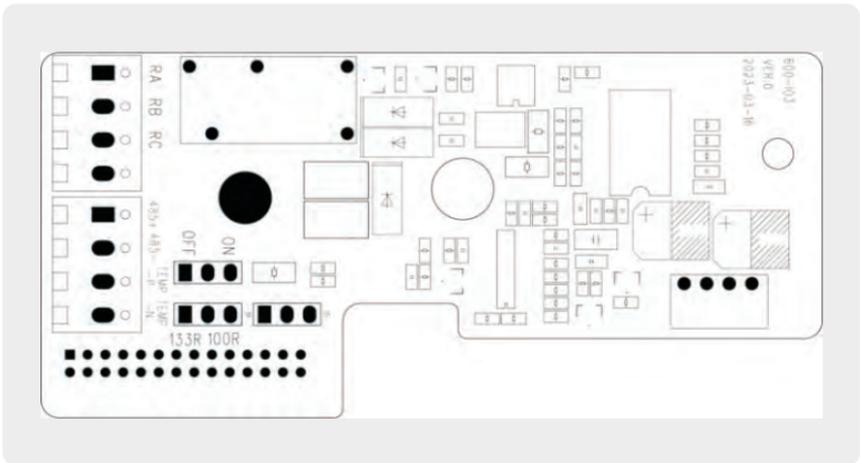
Figure 1-3 Appearance and layout diagram of I/O3 expansion card
