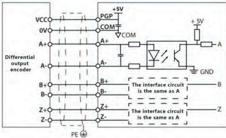
Figure 3-4 Differential output ABZ encoder card wiring diagram
