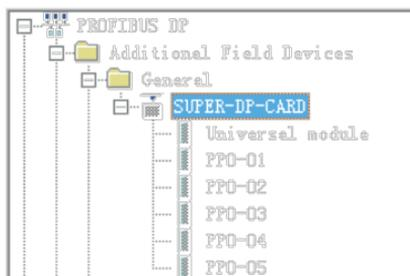
Note: If any master or slave station already exists on the HW config interface, the current interface needs to be closed when importing GSD. Click on the part marked by the red circle as shown in the following figure.
