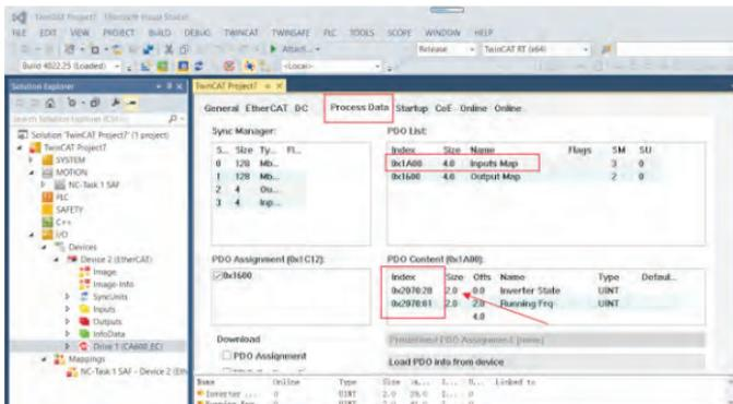
2. Configure RPDO. Select 0x1600 when configuring RPDO. The first two items are set to RPDO by default and cannot be changed. Right click on the location indicated by the red arrow in the following image to add RPDO mapping as needed.
