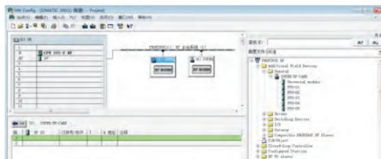
After adding the PPO type, you can see the address assigned by the PLC to the station, as shown in the figure. Slot 1 marked in the figure corresponds to the PKW address, with a total of 8 bytes, and slot 2 corresponds to the PZD address, with a total of 12 bytes.
