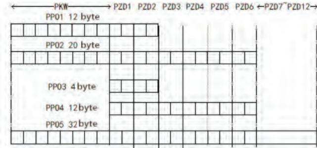
Figure 2-9 PPO type data format
