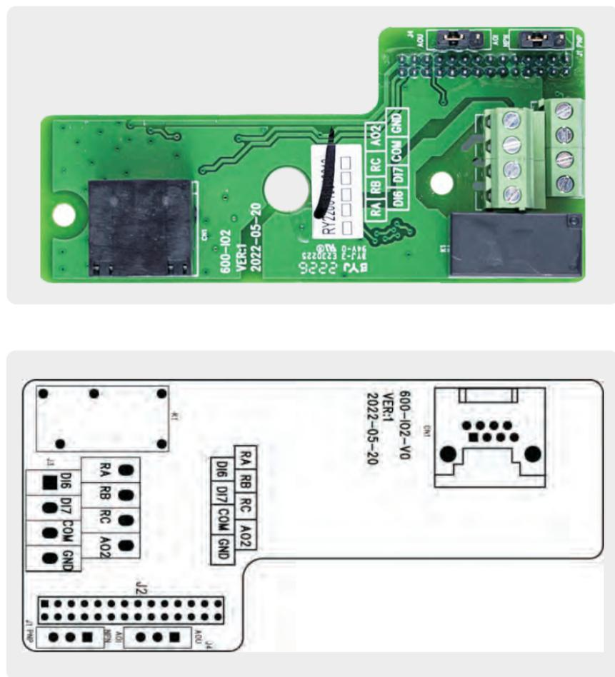
Figure 1-2 Appearance and layout diagram of I/O2 expansion card
