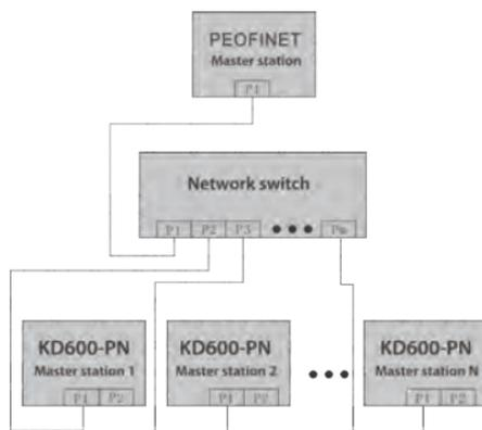
Figure 2-3 Star connection topology diagram
