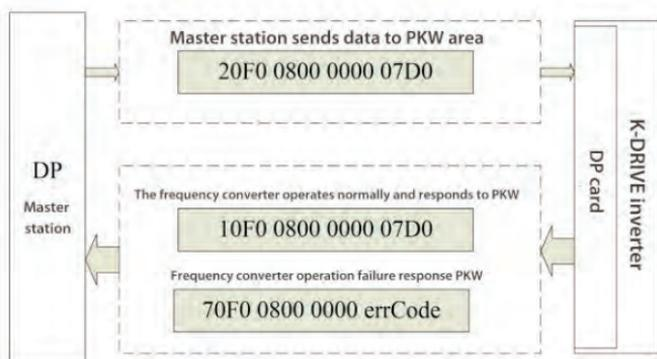
Figure 2-6 Example of master station reading frequency converter parameters and sending PKW data
