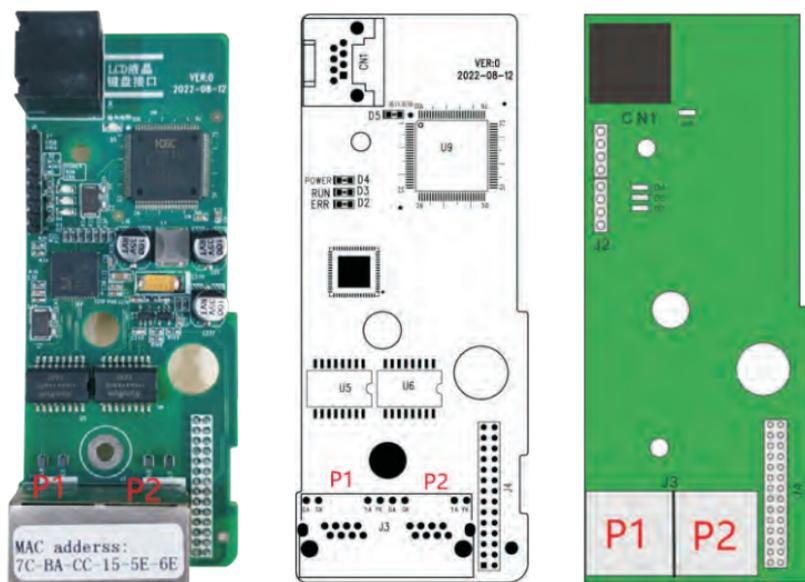
Figure 2-1 ProFinet Communication Card Appearance and Interface Layout
