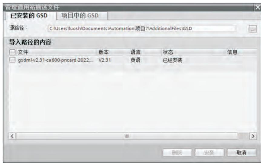
When the "Successfully Installed" interface appears, it indicates that you have clicked to close. After installing GSD, PORTAL will automatically close the configuration interface and complete the installation. You can find the device corresponding to the P\_PN in the hardware device tree, as shown in the following figure:
