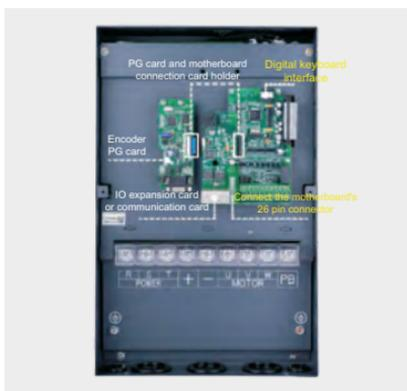
Installation diagram of 11KW and above models
