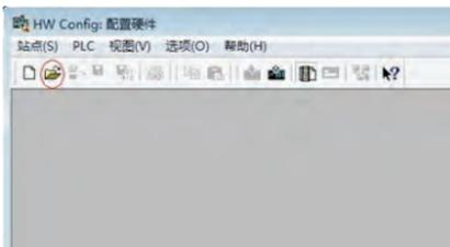
Select the previously closed configuration and click "Confirm" to open the original configuration.
