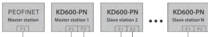
Figure 2-2 Bus type connection topology diagram
