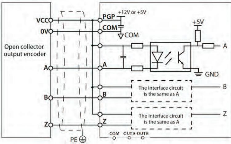
Figure 3-2 Open collector ABZ encoder card wiring diagram
