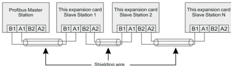
Figure 2-8 Schematic diagram of the connection between this DP expansion card and the Profibus master station
