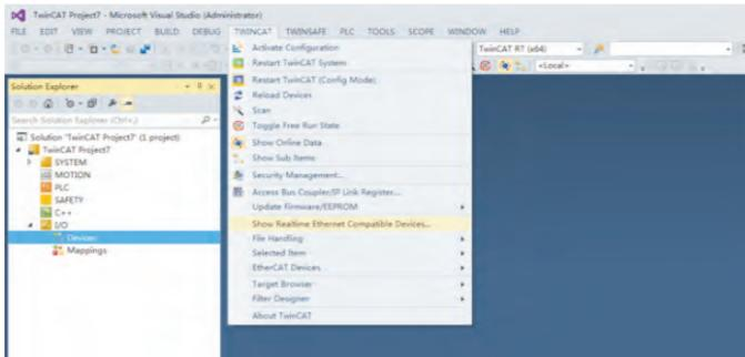
Select TWINCAT>Show Real Time Ethernet Compatible Devices. In the displayed dialog box, select the local network adapter from the incompatible devices, and then click Install. When installed later, the installed network adapter is displayed in "Devices Installed and Ready for Use".
